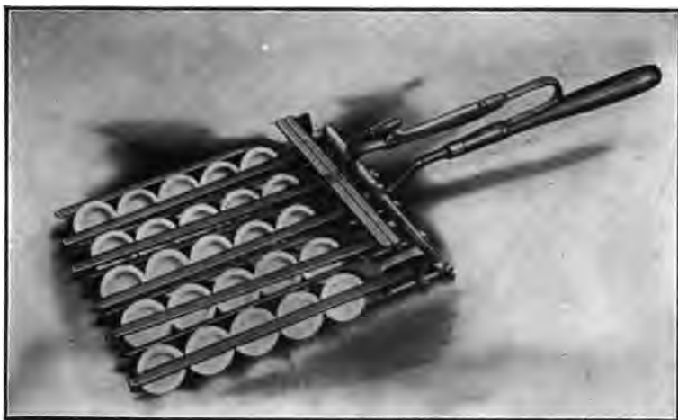
FIG. 27.—MULTIPLE SCORIFIER TONGS. (Keller.)
